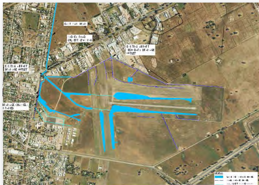
Figure 3.11 Benalla Airport Drainage Layout
